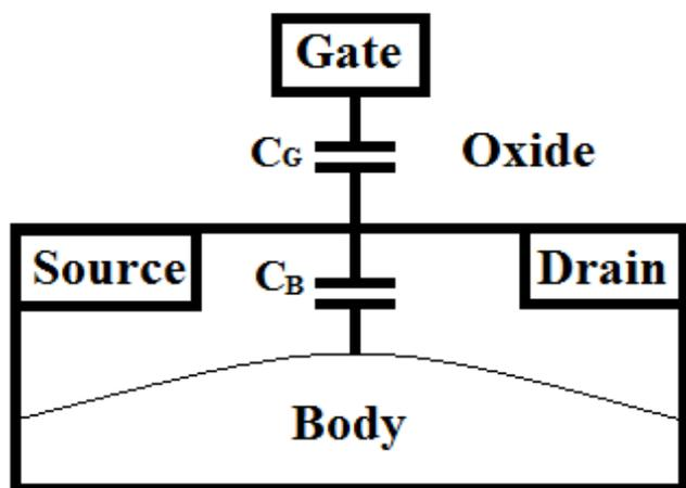
Fig. 2. Cross section of a long channel model
